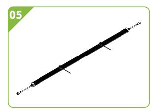
• Snap the lamp into the clip, the clip is 1ft away from the inner edge of the end cover.
