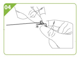
• Adjust the head position of the cable tie to the middle of the clip.
