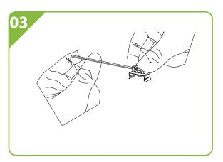
• The cable tie is passed through the other hole of the clip and through the lower hole of the cable tie.
