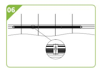
• Use cable ties to tie the fixtures horizontally to the brackets.
