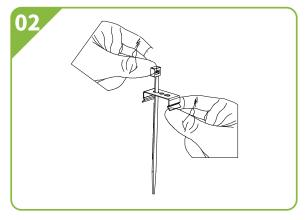
• Put the cable tie through the hole of the clip.
