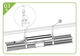
• Pass the hook through the mounting bracket and hang it on the hook of the lamp body so that the lamp body is parallel to the mounting bracket.
