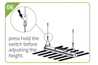
•Adjust the height by pull the cable.
