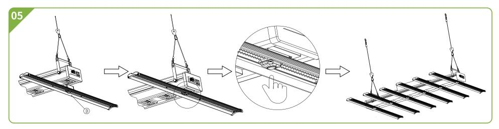
•Attach the light module to the chassis, press the button to lock.(Press again to remove the light module from the chassis.)
